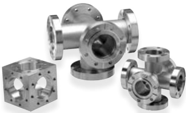
These fittings are manufactured with a flange on each end of a 5 or 6 sided tubing junction. These crosses accommodate complex junctions or alignment considerations for vacuum system design. Larger sizes are sometimes used as the starting point of a simple vacuum chamber design. **ANCORP** manufactures standard 5 and 6-way crosses and cubes in 304L stainless steel, other materials are available on request. Cubes are machined from a
