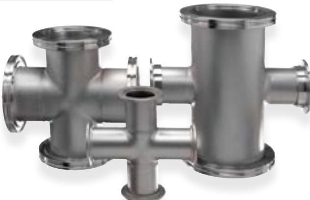
These fittings are manufactured with a flange on each end of an "X" shaped section of tubing. Crosses accommodate junctions or alignment considerations for vacuum system design. Crosses are also used as junction adapters between different tubing sizes or flange types. These fittings are available in all ISO sizes and flange types. **ANCORP** manufactures vacuum crosses in 304 stainless steel and aluminum.
