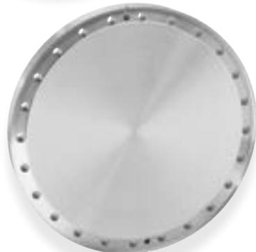
Female flanges accept the sealing gasket while the male flange has a protruding circular ridge that fits into the gasket groove on the receiving female flange. Standard wire seal blank flanges are manufactured of 304L stainless steel. Other materials are available on request.
