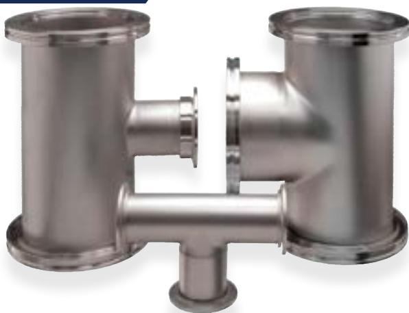
These fittings are manufactured with a flange on each end of a "T" shaped section of tubing. Tees accommodate junctions or alignment considerations for vacuum system design. Tees are also used as junction adapters between different tubing sizes or flange types. These fittings are available in all ISO sizes and flange types. **ANCORP** manufactures vacuum tees in 304 stainless steel and aluminum.
