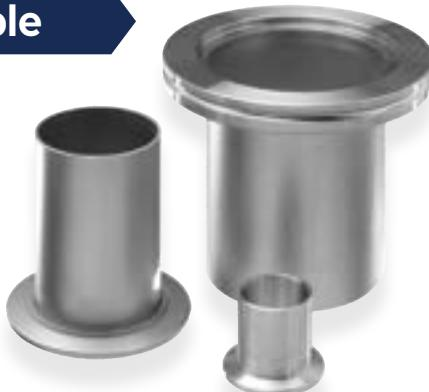
These fittings are manufactured with a flange on one end and raw tubing on the other. Half nipples are often welded onto a custom vacuum system or instrument by a customer with in-house welding capabilities. However, these fittings can also be used with quick connect compression fittings to make a vacuum tight connection without welding. **ANCORP** manufactures vacuum half nipples in 304 stainless steel and aluminum.
