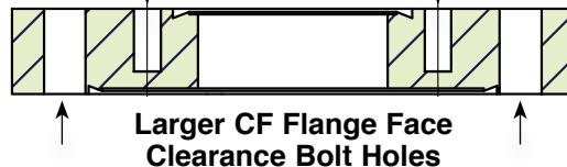
These flanges are manufactured with different size CF flange on either side of the flange. They allow direct assembly of two different sizes of CF flanges with minimal impact on the length added to your system to accomplish the transition. Zero-length reducers are the width of one standard flange.
