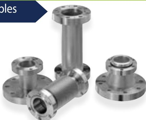
Nipples are manufactured with a flange on each end of a straight section of tubing. Nipples are used to create a weld free straight connection within a vacuum system. Nipples are also used as straight adapters between different tubing sizes or flange types. These fittings are available in all CF sizes and flange types. ANCOP manufactures standard nipples in 304L stainless steel, other materials are available on request.
