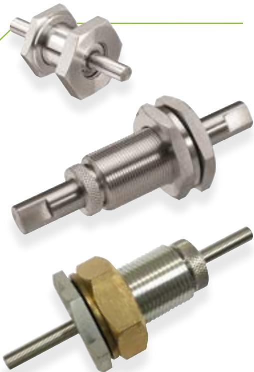
**ANCORP's** elastomer sealed rotary feedthrough is ideal for users requiring a rotary feedthrough for manual operation. The 1/4 inch shaft is supported by two ball bearings for smooth rotation. The 3/8 inch and 1/2 inch feedthroughs utilize bronze bearings to support the shaft. The shaft is sealed by a preloaded O-ring virtually foolproof! No spring to wear out or worry about.
