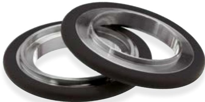
With our adaptive centering ring you can adapt directly from a QF10 to a QF16, QF20 to QF25 and QF32 to QF40. The connections can then be fastened with a standard clamp that corresponds with the larger of the two sizes. Adaptation to these standard sizes will greatly expand the number of components that have standard dimensions compatible with your vacuum system. This will ease your system assembly, decrease product delivery time and reduce cost.
