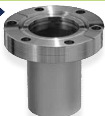
Half Nipples are manufactured with a flange on one end and raw tubing on the other. Half nipples are often welded onto a custom vacuum system or instrument by a customer with in-house welding capabilities. However, these fittings can also be used with quick disconnect compression fittings to make a vacuum tight connection without welding. ANCOP manufactures standard half nipples in 304L stainless steel, other materials are available on request.
