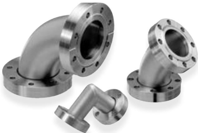
Elbows are manufactured with a flange on each end of a curved section of tubing. Elbows accommodate turns or alignment considerations for vacuum system design. Elbows are offered in four designs; 45° radius elbow, 90° radius elbow, 90° mitered elbow and 90° mitered high conductance elbow to accommodate a wide variety of system configurations. **ANCORP** manufactures standard Elbows in 304L stainless steel, other materials are available on request.
