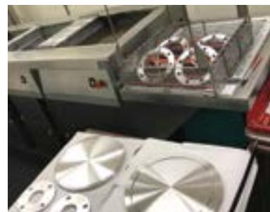
After cleaning and testing, flanges and small components are hermetically sealed in vacuum board packaging and are ready for UHV installation. Larger flanges are covered with a layer of foil and protective plastic shields. Weldments and assemblies are then bagged, bubble-wrapped, and inserted into a shipping container surrounded by void filling "pillow" wrap. Custom crating is available.
