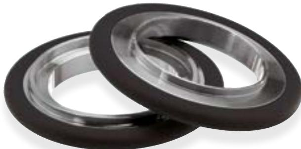
These sealing assemblies allow you to adapt directly from the rarely used ISO-QF sizes (QF10, QF20 and QF32) to commonly available ISO-QF sizes (QF16, QF25 and QF40). The adapted assembly can then be fastened with a standard clamp that corresponds with the larger of the two sizes.
