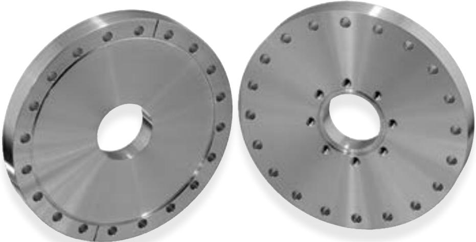
**ORDERING NOTE:** When ordering hardware for your Zero Length Reducer take note of the flange bolt holes to order clearance bolts kits and tapped bolt kits appropriate to the design of your flange. "T1" and "T2" designate one or both sets of bolt holes are tapped. The smaller flange is always tapped. Zero Length Reducers are only the width of 1 standard CF flange.
