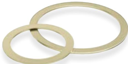
The basic seal for the CF flange system is an oxygen free electronic grade (OFE) copper gasket that is compressed between the knife-edges (flat version) or between a male and female edge (round single strand version) of two CF flanges to create a seal capable of achieving ultra high vacuum pressures. Copper gaskets have a temperature range of -200°C up to 450°C.
