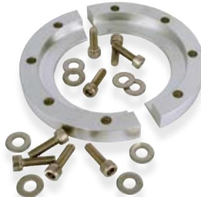
Bulkhead clamps are used to fasten ISO-QF style flanges and components directly to valves, chamber walls, baseplates or bulkheads. The object to which the flange is sealing must have a compatible bolt hole pattern and sealing groove machined into the sealing surface.
