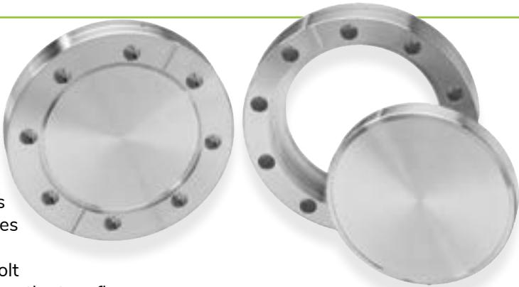
Fixed and rotatable flanges have two bolt hole options: clearance or tapped bolt holes. Clearance bolt holes allow for unrestricted passage of a bolt through the flanges. The bolt is then tightened with a nut on the back side of the flange assembly. Tapped bolt holes are threaded to receive and tighten the bolt directly and do not utilize a nut. Standard CF blank flanges are manufactured of 304L stainless steel. Other materials are available on request.
