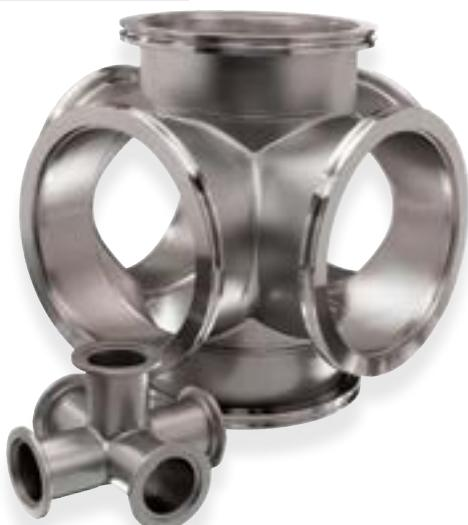
These fittings are manufactured with a flange on each end of a 5 or 6 sided tubing junction. Crosses accommodate complex junctions or alignment considerations for vacuum system design. Larger sizes are sometimes used as the starting point of a simple vacuum chamber design. **ANCORP** manufactures 5 and 6-way vacuum crosses in 304 stainless steel and aluminum.
