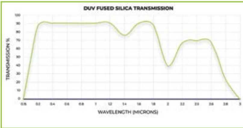
**Zero-length DUV grade fused silica viewports** are available in a variety of ConFlat (CF) flange sizes for ultra-high vacuum (UHV) performance. Single AR and broadband AR anti-reflective coatings are available for minimized reflectance.
