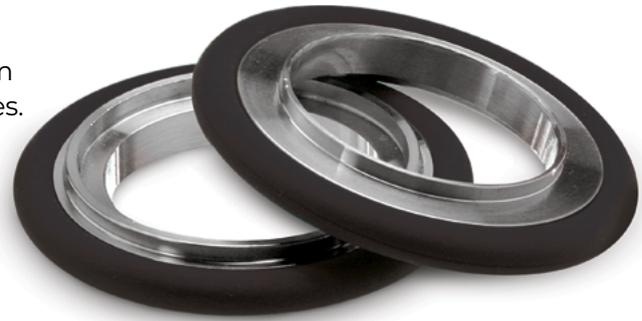
With our adaptive centering ring, you can adapt directly from a QF10 to a QF16, QF20 to a QF25, and QF32 to a QF40. The connections can then be fastened with a standard clamp that corresponds with the larger of the two sizes. Adaptation to these standard sizes will greatly expand the number of components that have standard dimensions compatible with your vacuum system. This will ease your system assembly, decrease product delivery time, and reduce cost.
