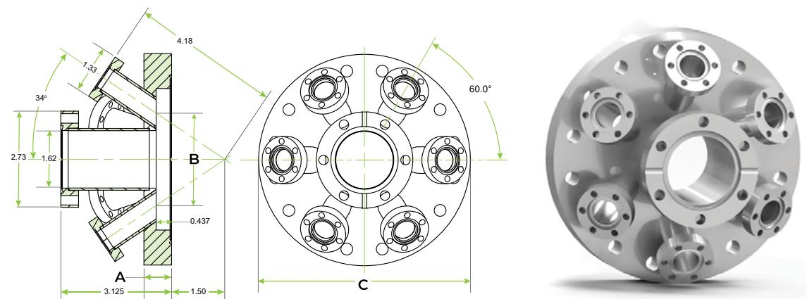
CF600 (6") or CF800 (8") O.D. multiport flange with (1) CF275 (2.75") fixed center flange on tube extension and (6) CF133 (1.33") fixed mini flanges angled-in on tube extensions, focused on a target point.
