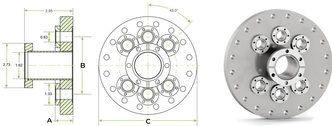
CF600 (6") or CF800 (8") O.D. multiport flange with (1) CF275 (2.75") fixed center flange on tube extension and (6) CF133T (1.33", tapped bolt holes) fixed mini flanges, flush-mounted.
