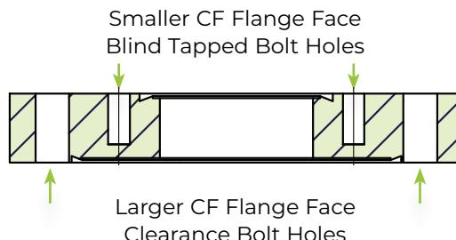
CF double-sided flanges allow direct assembly of two different sizes of CF flanges with minimal impact on the length added to your system to accomplish the transition. Zero-length reducers are the width of one standard flange.
