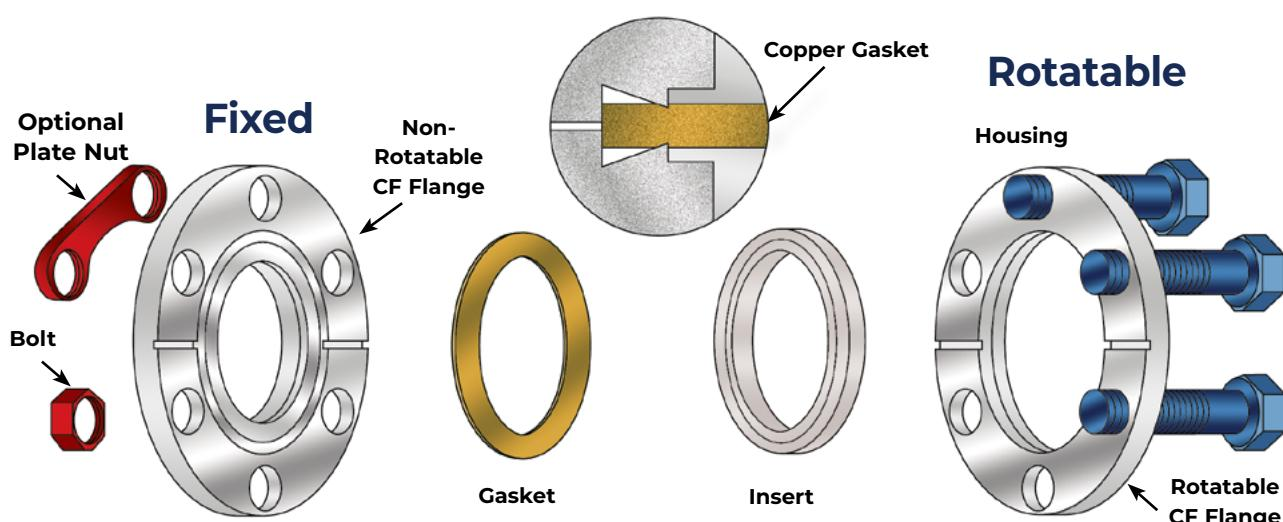
The CF flange system provides a complete range of flanges to mount with tubing sized 3/4 inch up to 14 inches in diameter. The CF seal assembly consists of three sub-components: two flanges, a sealing gasket, and a fastener to compress the seal between the two flanges.
